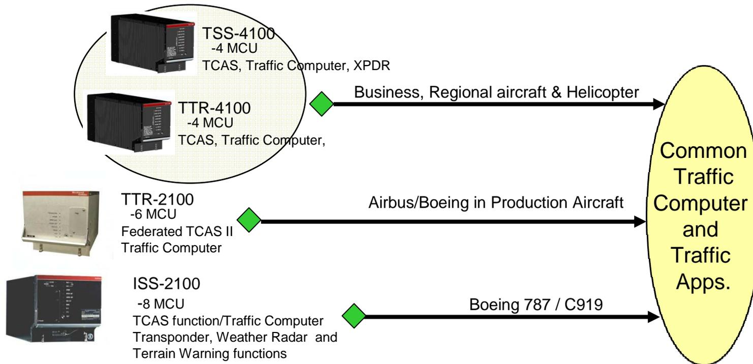
Common Traffic Computer Design enables re-use of ADS-B In Applications
